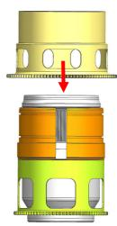
4. Insert the STE2875-Z Zoom Gear on the plastic C-ring for zoom until it reaches the flange of the plastic C-ring.
