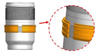
1. Insert the plastic C-ring for focus as shown and place it over the lens
