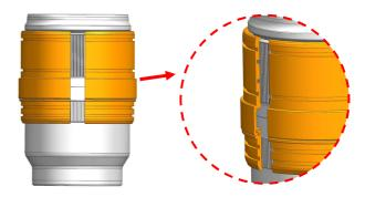
2. Insert the plastic C-ring for zoom as shown and place it over the lens, then lock the zoom c-ring as shown.
