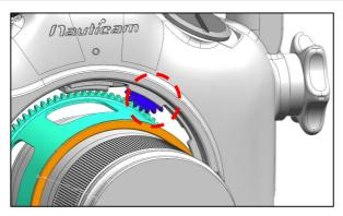
1. The STE2875-F Focus Gear can be controlled by zoom/focus knob of the housing.
